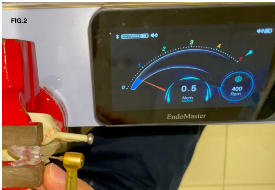
Figure 2. Video recording the torque values during instrument progression inside canal
